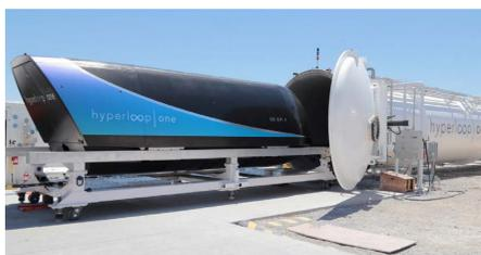
Currently in development as an experimental transportation method, the Hyperloop connects two destinations with a sealed tube that transports passenger pods at high speeds. A hyperloop network would connect regional destinations similar to a rail network.
